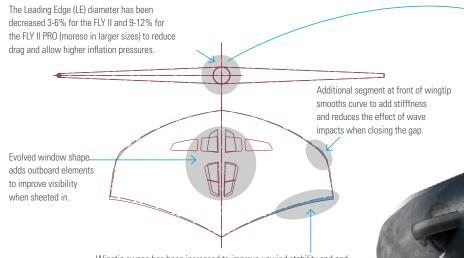
Wingtip sweep has been increased to improve upwind stability and and for more control while holding the wing in a neutral position. The pointing ability is improved due to moved Center of Effort slightly to the leech.
